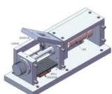
In heating system of TX500D, temperature sensor is mounted on the air that surrounds sample tube and the tube is heated via air, which improves heating efficiency and coincidence between control temperature and actual temperature.
